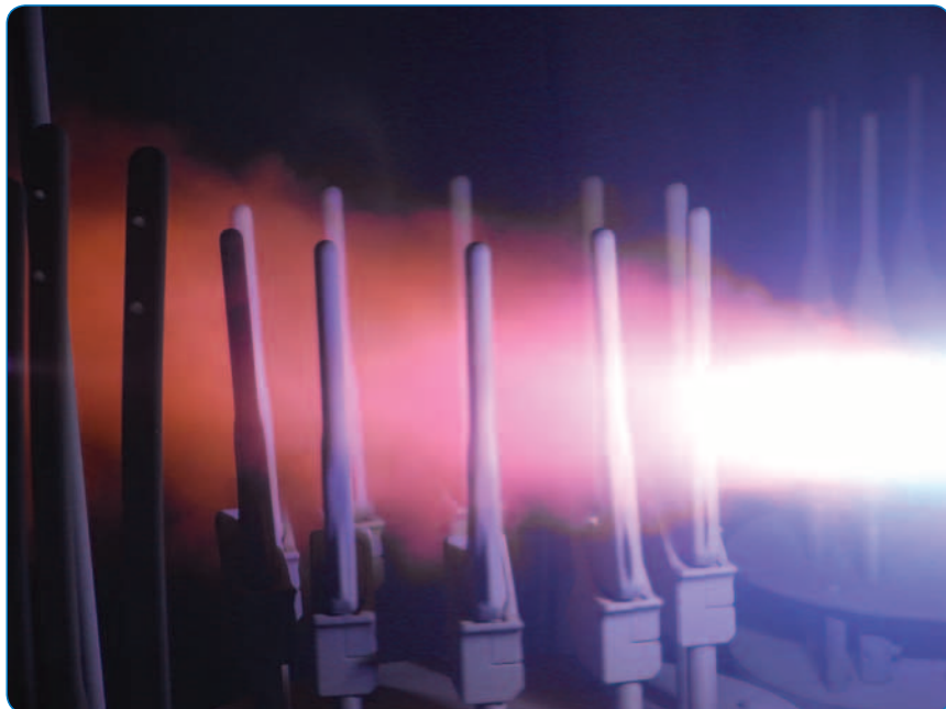
Fig.1 H-A.C. coating application using a plasma torch at 20,000°C.
